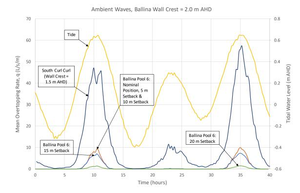
Figure 9.5 Overtopping for Pool position 3 (wall at 2.0 m AHD), ambient waves
