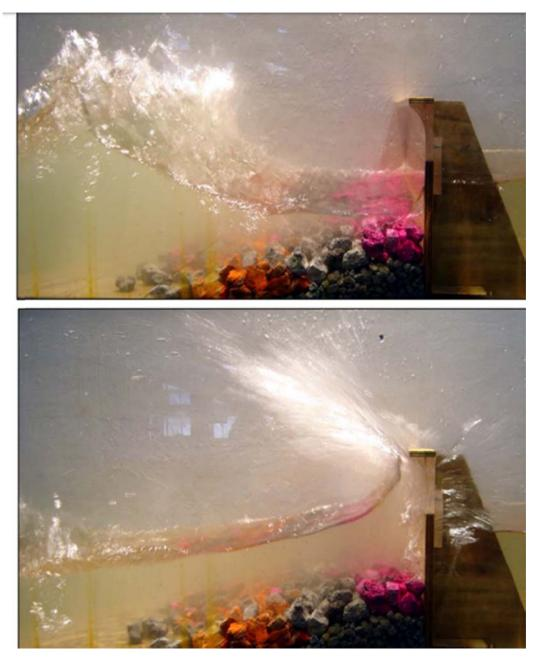
Figure 6.4 Curved wave deflector wall physical model
