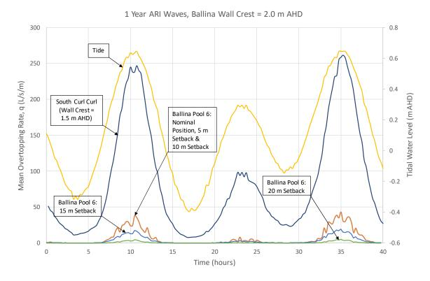
Figure 9.7 Overtopping for Pool position 3 (wall at 2.0 m AHD), 1 year ARI waves
