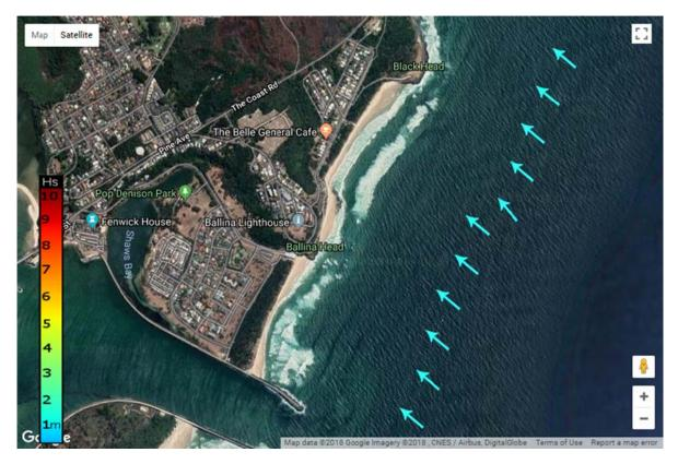
Figure 4.4 Wave transformation to 10 m contour with NSW coastal model
