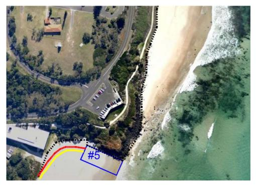
Notes: Black dashed line is present 2 m AHD contour based on optical drone survey by WRL on 8/8/2018; Yellow dashed is with pool under ambient conditions; Red is post-storm. Existing and future armouring may modify these.
