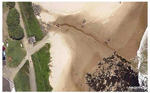
Figure 4.12 Stormwater outfall with accreted beach (Source: NearMap)
