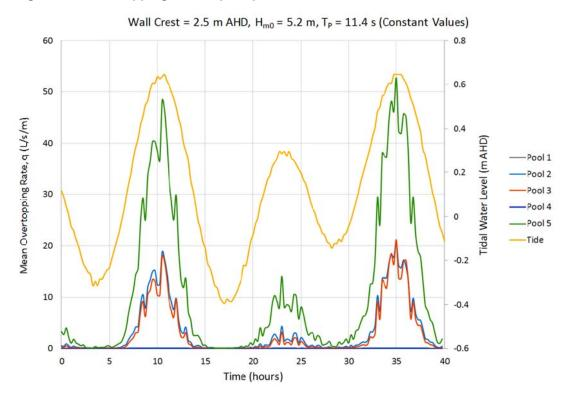
Figure 7.13 Overtopping Ballina pool positions 1 year ARI waves, wall at 2.5 m AHD
