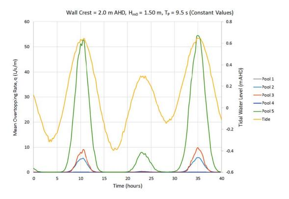
Figure 7.8 Overtopping Ballina pool positions ambient waves, wall at 2.0 m AHD
