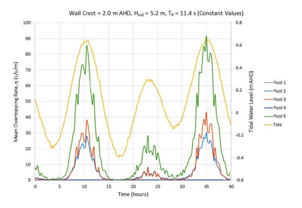
Figure 7.10 Overtopping Ballina pool positions 1 year ARI waves, wall at 2.0 m AHD
