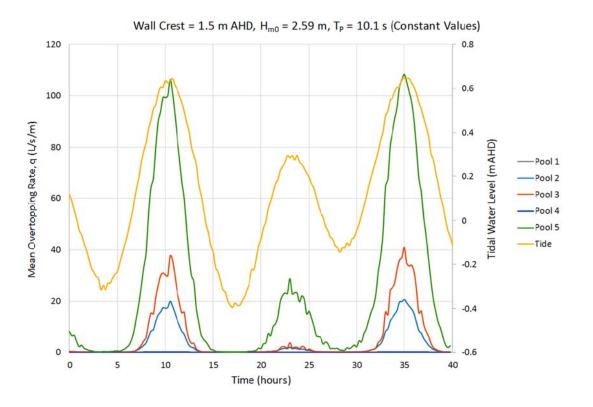
Figure 7.6 Overtopping Ballina pool positions 10% exceedance waves, wall at 1.5 m AHD
