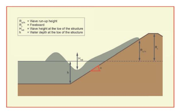
Figure 6.1 EurOtop cross section for overtopping
