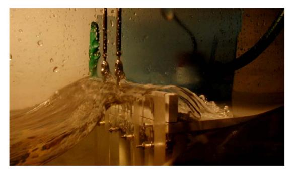
Figure 6.2 Wave overtopping physical model
