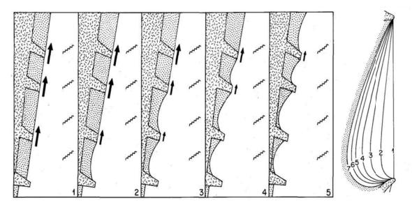
Source: Stephens et al., (1981) Figure 4.15 Coastal evolution and headland bypassing on a littoral drift coast
