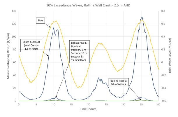
Figure 9.9 Overtopping for Pool position 3 (wall at 2.5 m AHD), 10% exceedance waves
