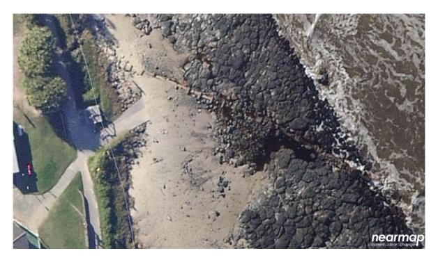
Figure 4.11 Stormwater outfall with eroded beach (Source: NearMap)
