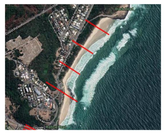
Figure 4.17 Photogrammetry transects (P1 at south of Shelly Beach, P4 at north)
