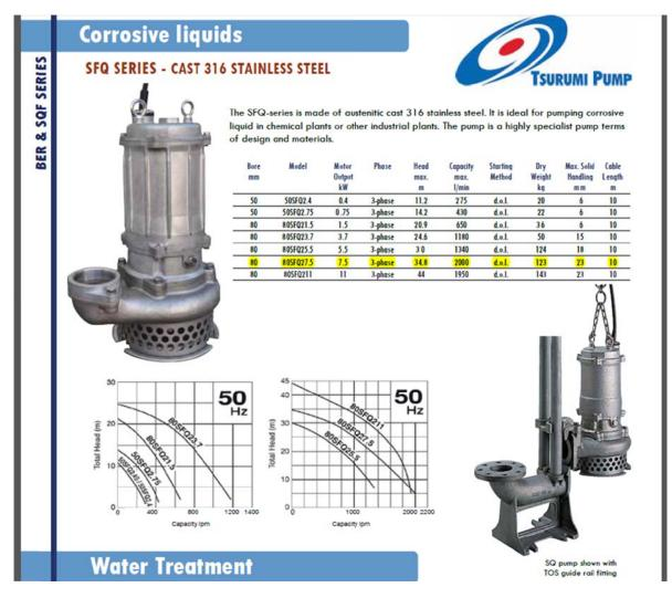
Figure 5.5 Tsurumi pump details
