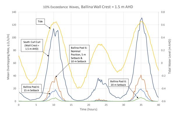
Figure 9.3 Overtopping for Pool position 3 (wall at 1.5 m AHD), 10% exceedance waves
