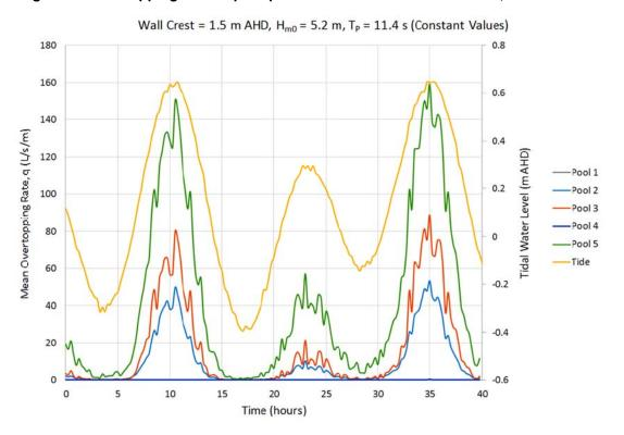
Figure 7.7 Overtopping Ballina pool positions 1 year ARI waves, wall at 1.5 m AHD
