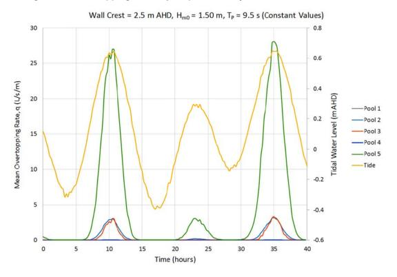
Figure 7.11 Overtopping Ballina pool positions ambient waves, wall at 2.5 m AHD
