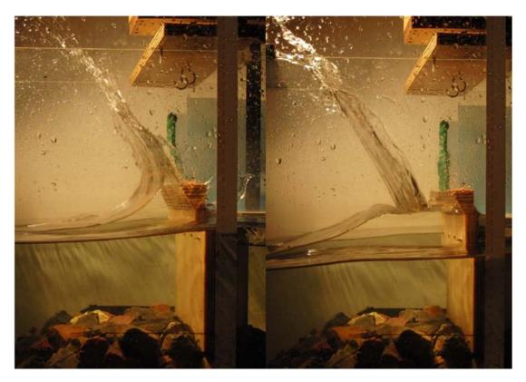
Figure 6.3 Angled wave deflector wall physical model
