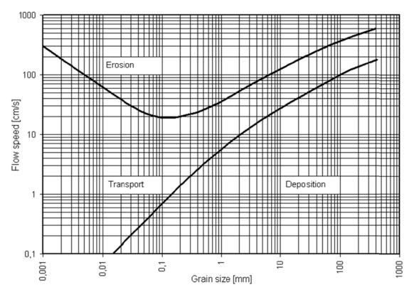
Figure 5.7 Hjulstrom diagram for sand erosion
