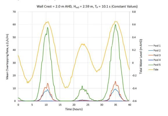
Figure 7.9 Overtopping Ballina pool positions 10% exceedance waves, wall at 2.0 m AHD
